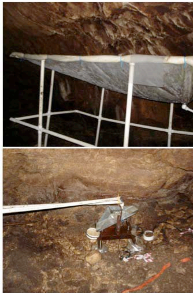
Figure 5. Drip collector and tipping bucket used for measuring cave recharge..
