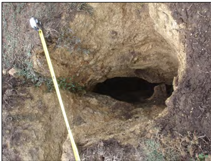
Figure 3-1. (top) Julie Jenkins stands in Horseshoe Sink. (Bottom) Horseshoe Sink on Dec 13, 2007. A single aperture into the Georgetown Limestone was open at that time. Since 2013, five similar apertures have opened after flood events.
