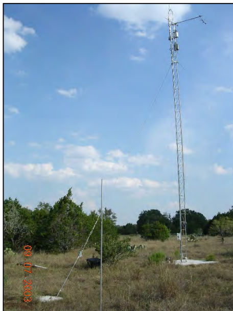
Eddy covariance tower installed on CoA J17 WQPL as cooperative recharge study with University of Texas Department of Geosciences from 2002 to 2009. Measured parameter included precipitation, runoff, evapotranspiration, and soil moisture.
