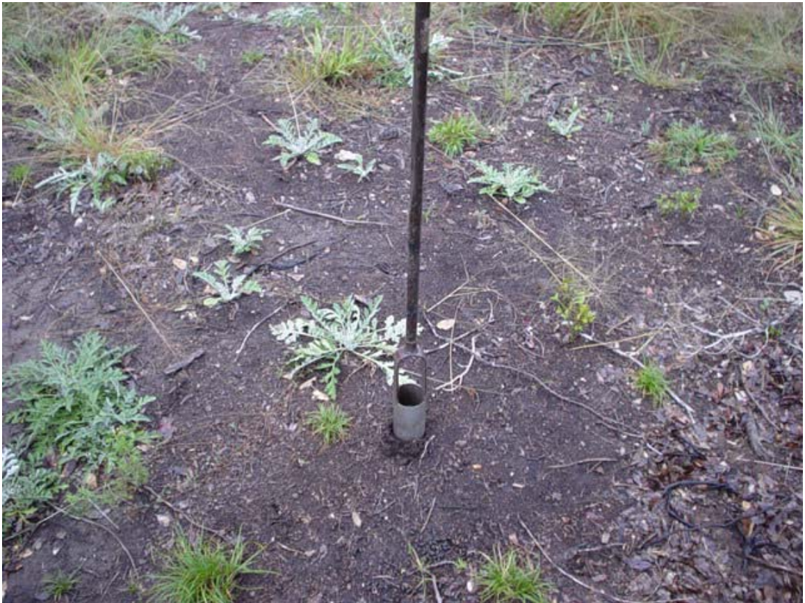
Figure G.6. Soil auger used to take soil samples.
