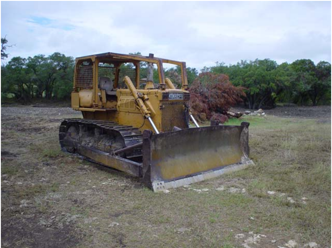
Figure G.7. Crawler tractor used to clear juniper.
